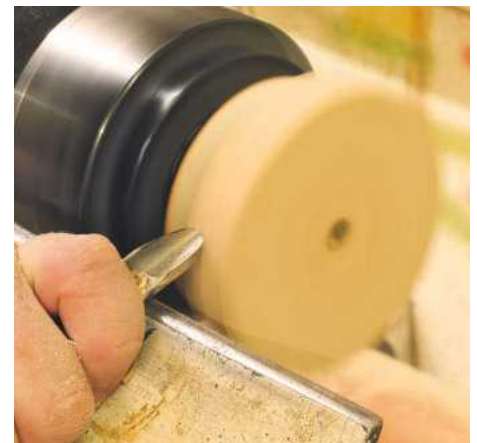
▲ Pic.9 Once mounted on the screw chuck, make it round with the spindle or bowl gouge. Work away from the back surface so you don't get any breakout on the underside
